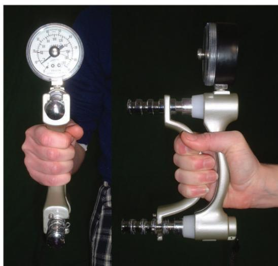
**Figure 1.** Front and side views of a Jamar dynamometer being used on position-2.
