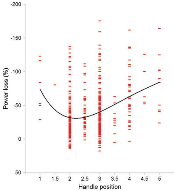
**Figure 8.** Power loss in all injured hands and the calculated polynomial trend line for each Jamar handle position demonstrating increased loss of power associated with maximum grip occurring at positions other than 2 and 3 ( $R = 0.34$ ,  $p < 0.001$ ).
