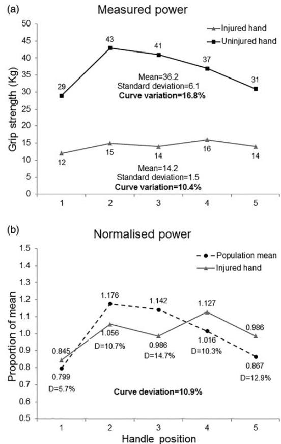
**Figure 3.** (a) The grip strength at the five positions of both hands of a male claimant plotted showing the power exerted at each handle position. The method of calculation of the curve variation score is shown. (b) The normalised curve for the injured hand is plotted and compared with the mean values for the male population. The method of calculation of the curve deviation score is shown.
